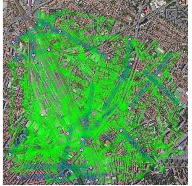
Figure 4: A sample dense scenario with 20 UAVs flying over a 2km x 2km urban area. UAVs are represented as circles (with their current speed vector). 4D contracts (and their respective safety tubes) are represented in green. Current segments are represented in blue.
