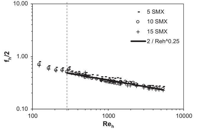
**Fig. 3.**  $f_h/2 = f(Re_h)$  for the SMX mixer with  $n_e = 5; 10; 15$ .
