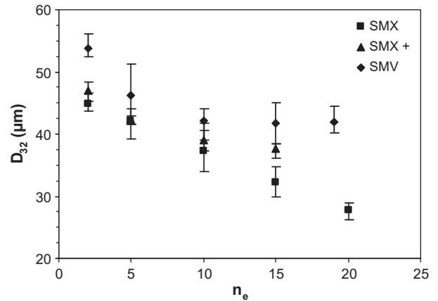
**Fig. 15.** Influence of the number of elements on the Sauter diameter for the three designs with  $Q_{tot} = 335$  L/h.
