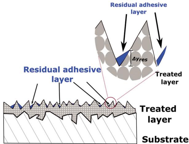
**Figure 23.** Residual adhesive layer interlocked into the asperities.
