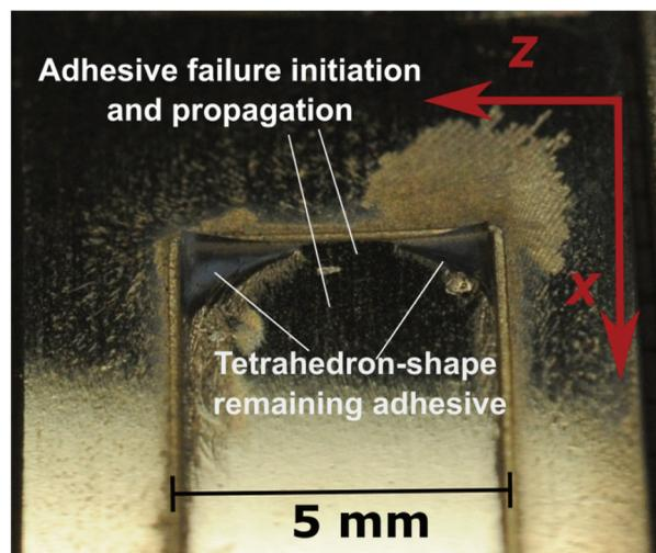
**Figure 10.** Adhesive failure initiation and propagation obtained for the configuration P4000 + diamond paste –No small round area is tracked, although a similar fracture shape is obtained (see Figure 9 -a).
