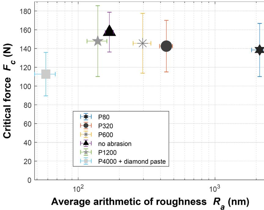
**Figure 8.** Critical force versus average arithmetic of roughness.
