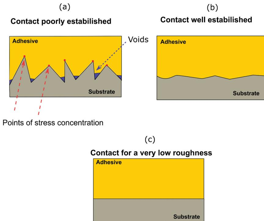
**Figure 1.** Region of intimate contact between adhesive/substrate.
