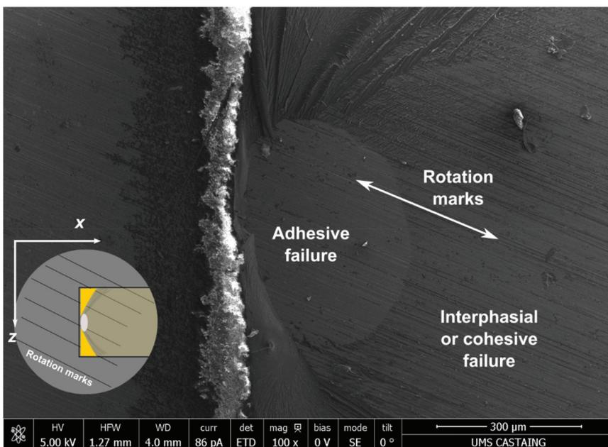
Figure 12. SEM of adhesive failure initiation –P1200.
