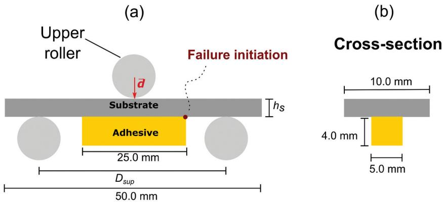
**Figure 2.** Dimension of 3PBT according to ISO 14679.<sup>[11]</sup>.
