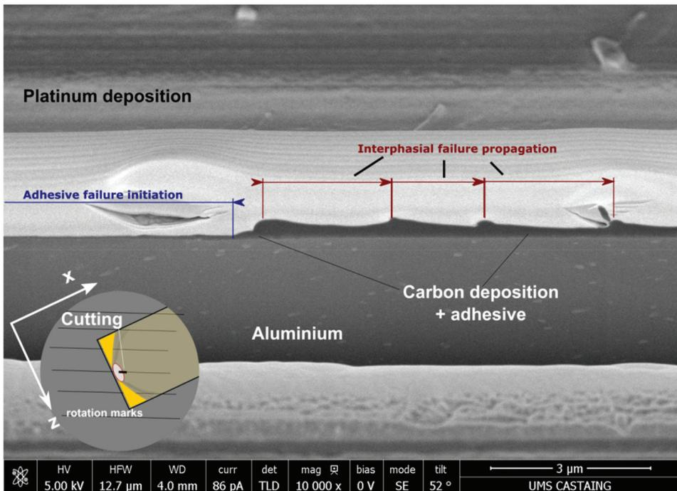
**Figure 14.** Adhesive-to-interphase transition failure along a valley.
