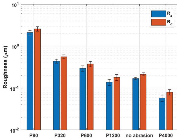
Figure 4. Roughness evaluation using different abrasive papers.
