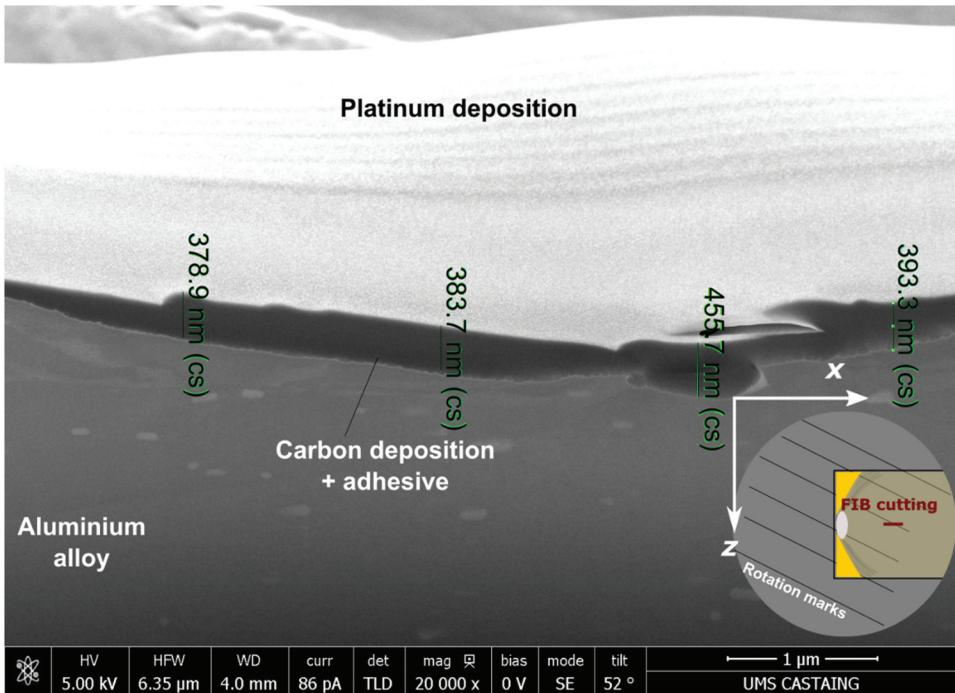
**Figure 19.** FIB cutting across interphasial failure propagation—a variation of the residual adhesive thickness into a roughness valley.
