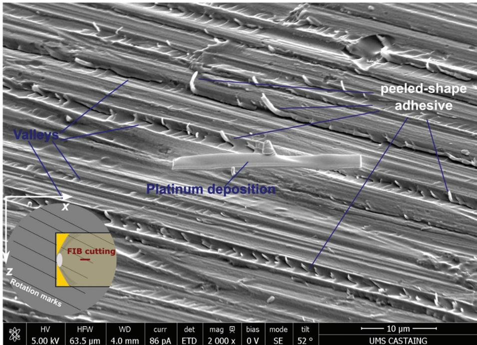
**Figure 17.** SEM of a post-mortem interphasial failure propagation and the analyzed region via FIB (P1200).
