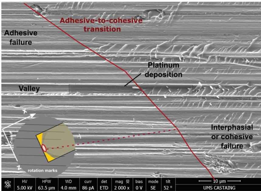
**Figure 13.** Cutting process along a rotation mark (valley) performed via Focused Ion Beam (FIB) milling (Ga<sup>+</sup> ions). -P1200.
