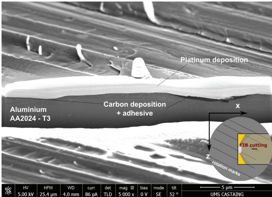
**Figure 18.** A FIB cutting across interphal failure propagation–adhesive interlocked mostly at roughness valleys.
