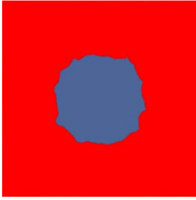
Fig. 4. Top view of the instantaneous numerical open eye, obtained at Q = 0.6\text{ l/min} . The numerical results are obtained with a minimum grid size of \Delta x = 527\ \mu\text{m} and the oil interface is colored in red.
