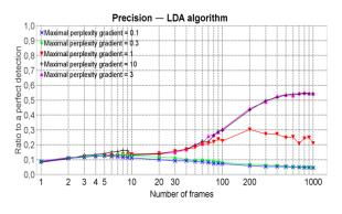
Fig. 32. Precision of the LDA algorithm relative to the trace size and parameterized by maximal perplexity gradient
