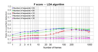
Fig. 31. F score of the LDA algorithm relative to the trace size and parameterized by the number of keywords
