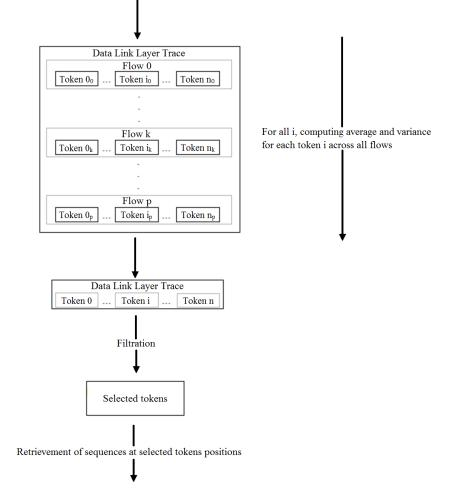
Fig. 3. Illustration of the VDV algorithm applied to our study case
