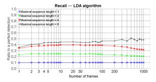
Fig. 27. Recall of the LDA algorithm relative to the trace size and parameterized by maximal sequence length
