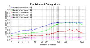
**Fig. 29.** Precision of the LDA algorithm relative to the trace size and parameterized by the number of keywords
