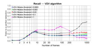
Fig. 15. Recall of the VDV algorithm relative to the trace size and parameterized by the filtration threshold value
