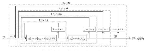
Fig. 8. Algorigram of the Gibbs sampler procedure
