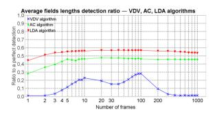
Fig. 44. Best average fields lengths detection ratio of the algorithms VDV, AC, and LDA
