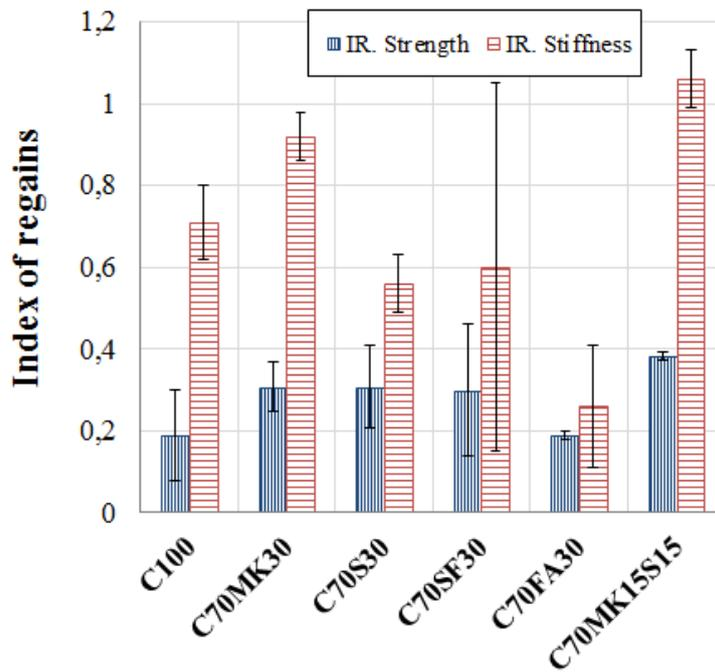
475 **Fig.10** Effect of different minerals additions on mechanical properties: index of stiffness
