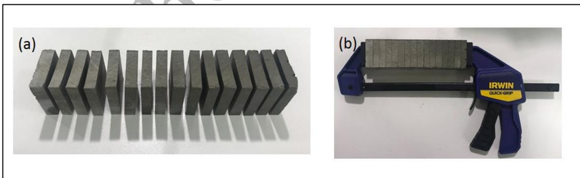
**Fig.3** Slices cut from 40x40x160 mm cement paste specimen (a), slices pressed together using a clamp (b).
