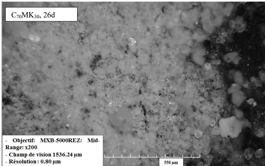
275 **Fig.4** 2D microscopic image of specimen with minerals additions before healing (48
