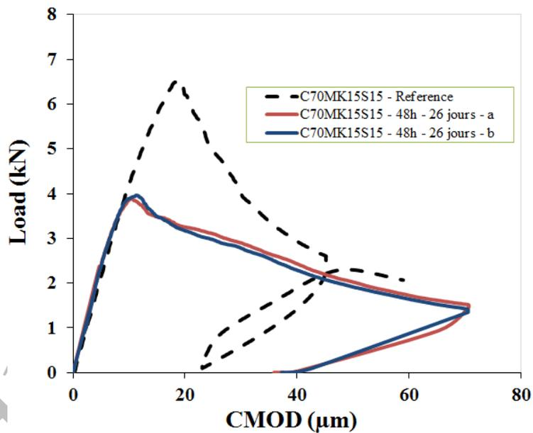
470 **Fig.9** Mechanical behaviour of aged mortar specimens for different SCM's mixtures (load
