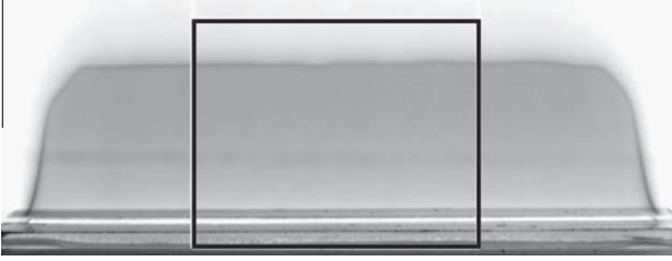
Fig. 3. Side view of the flame (photo of the experiment at \phi = 0.8 ). The rectangular box corresponds to the zone where the measurements of flame length are performed.
