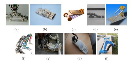
Fig. 3. Robotic feet with multiple segments structure or with soft structure (a) PNEUMAT-BB [52], (b) WABIAN-2R (multi-joint mechanism) [53–55], (c) [56], (d) [57], (e) [58], (f) [59], (g) KENGORO [60–62], (h) [63], (i) SoftFoot [64].
