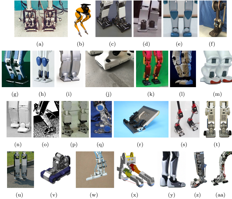
Fig. 2. Robotic feet with a one segment structure, with one segment with a wheel or with two segments structure (a) WL-12RVII [5, 6], (b) CASSIE [7, 8], (c) WABIAN-2R (unique-segment mechanism) [9], (d) BHR-2 [10–12], (e) HRP-2 [13, 14], (f) WALK-MAN [15], (g) P2 [16], (h) HRP-4 [17, 18], (i) KHR-3 [19, 20], (j) PYRENE (TALOS) [21], (k) JAXON [22], (l) VALKYRE [23, 24], (m) NAO [25–28], (n) ASIMO [29, 30], (o) Ken [31], (p) ROBIAN [32, 33], (q) iCub [34], (r) WABIAN-2R (two-segments mechanism) [35], (s) [36–40], (t) DRC-HUBO+ [41], (u) H6 [42, 43], (v) UT- \mu 2 [44], (w) BIPMAN [45], (x) PNEUMAT-BH [46, 47], (y) HRP-4C [48], (z) ARMAR-4 [49], (aa), LOLA [50, 51].
