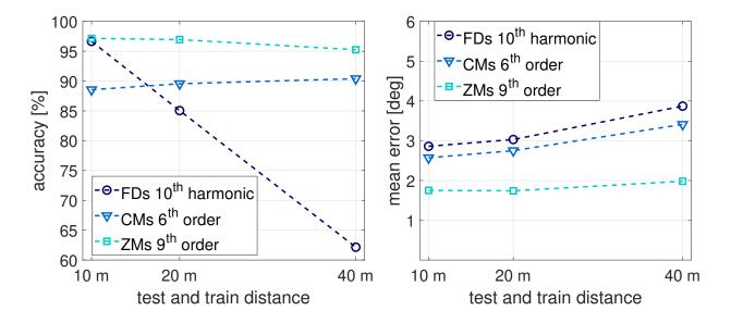
Fig. 6. Effect of a variation in the resolution of both the test and the training images ( $d_{test} = d_{train}$ ).
