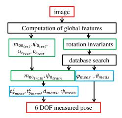
Fig. 2. Structure of the proposed pose estimation algorithm.
