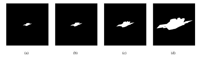
Fig. 4. Silhouette of the target satellite at 40 m (Fig.4(a)), 30 m (Fig.4(b)), 20 m (Fig.4(c)), 10 m (Fig.4(d)), for a  $1024 \times 1024$  pixel camera with FOV of  $30^{\circ}$ . The attitude of the S/C is  $\varphi = 70.41^{\circ}$ ,  $\vartheta = 66.92^{\circ}$ ,  $\psi = -29.58^{\circ}$
