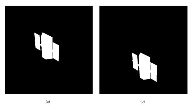
Fig. 8. Silhouette of the target satellite at 20 m, at a relative attitude of  $\vartheta=-35.02^\circ$ ,  $\psi=87.99^\circ$ . In Fig.8(a) the pointing error is  $\Delta\gamma=1.43^\circ$ , in Fig.8(b) it is  $\Delta\gamma=5.85^\circ$ .
