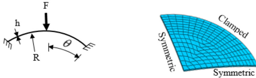
Figure 4. Description of spherical cap test
