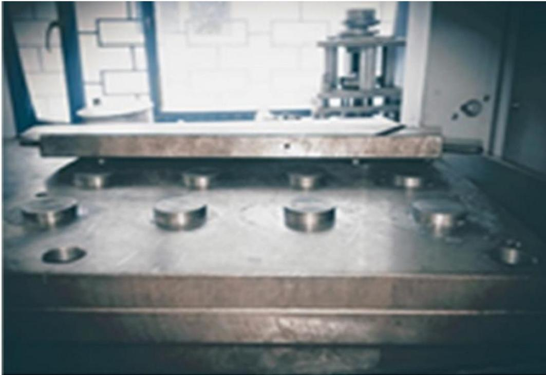
**Figure 2.** The used mould die for the briquetting process.
