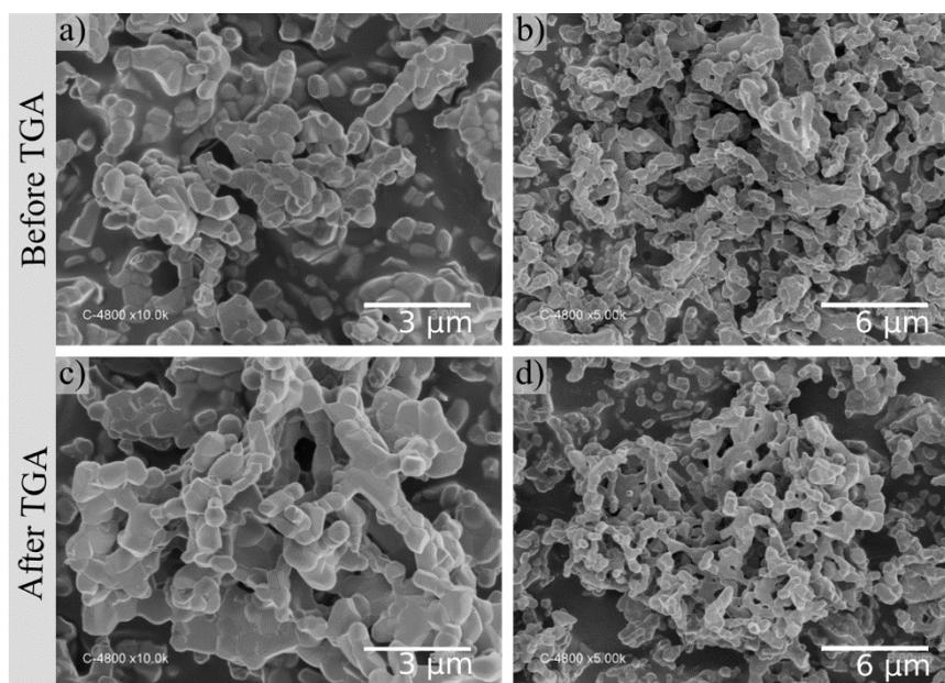
Figure 3: FESEM observations of LSMMg-P1 powder: a) and b) before cycling; c) and d) after cycling in TGA for CO<sub>2</sub> splitting
