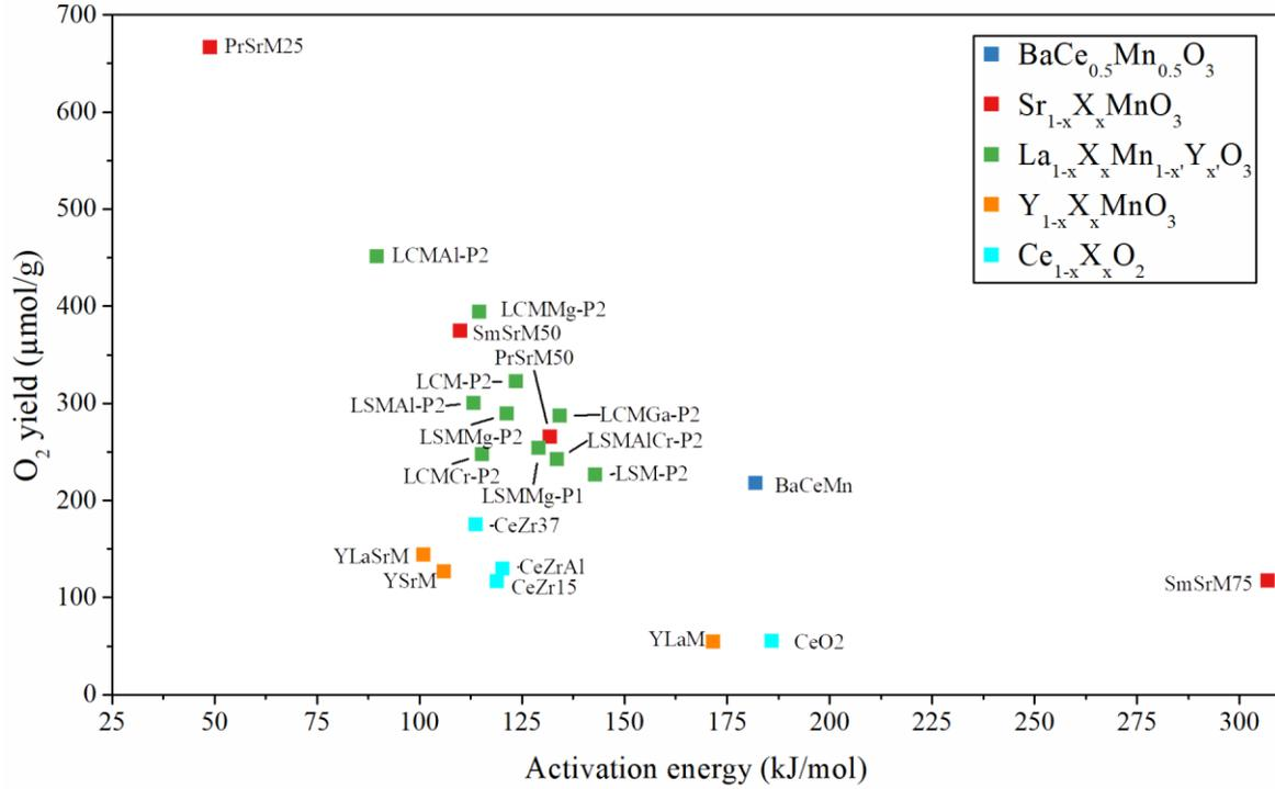
Figure 12: Experimental O<sub>2</sub> yield as a function of activation energy for the series of investigated reactive materials
