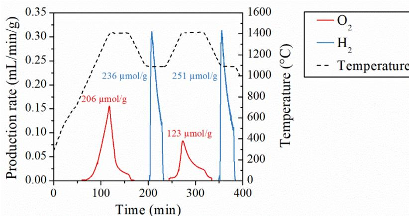
Figure 2: O<sub>2</sub> and H<sub>2</sub> production rates during two consecutive thermochemical cycles for H<sub>2</sub>O splitting, performed in a tubular furnace with LSMMg-P1
