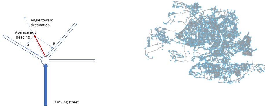
Fig. 3. Left: Illustration of steps of the randomized geo-routing algorithm. The traveller enters the intersection via the large blue arrow. Right: the map of Kaliningrad.
