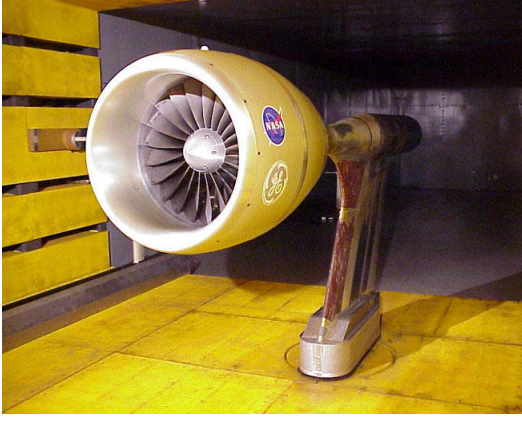
Figure 1: NASA SDT model installed in the NASA Glenn Wind Tunnel
