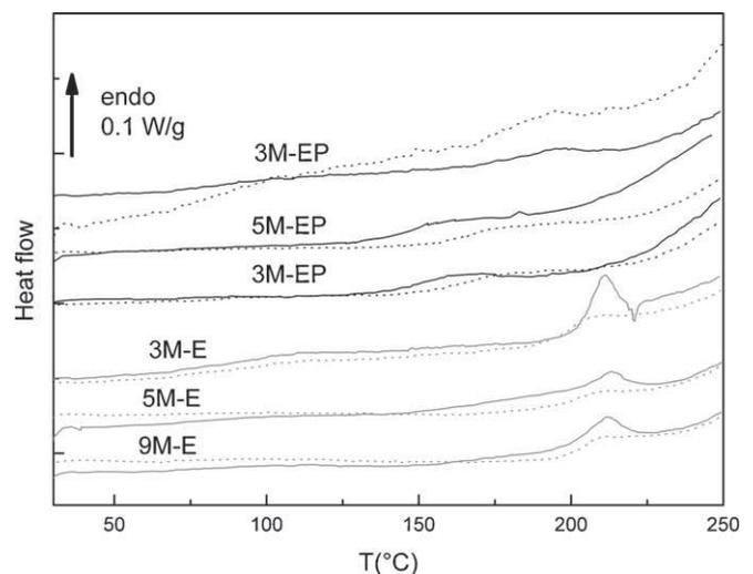
**Fig. 1.** Differential Scanning Calorimetry thermograms (2<sup>nd</sup> scans in solid line and 3<sup>rd</sup> scans in dot line) of elastin (E) and elastin-proteins (EP) fractions from children thoracic aortas.
