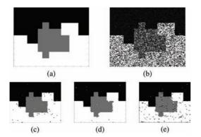
Fig. 4. (a) True labels, (b) observations, MAP label estimates for (c)  $\beta = 1$ , (d)  $\beta = 1.2$ , and (e)  $\beta = 0.8$ .
