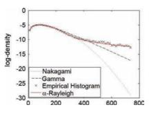
Fig. 7. Comparison of the B-mode histogram obtained from forearm dermis, and the corresponding estimations using the Nakagami, Gamma, and  $\alpha$  Rayleigh distributions. Plots presented in logarithmic scale to illustrate fitting at the tails.
