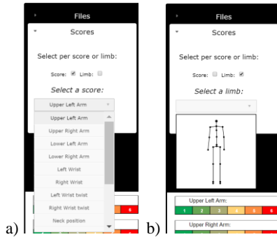
Figure 5: Selection of the RULA scores to visualise: a) Scores dropdown list, b) Skeleton sketch for joint selection
