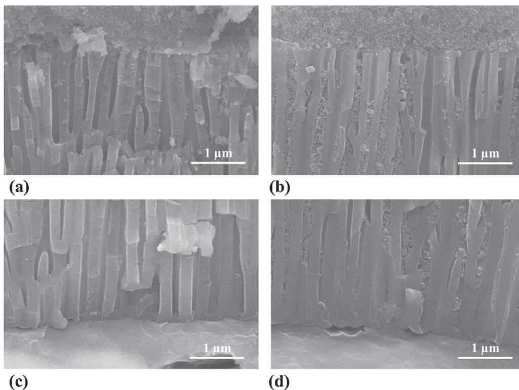
Fig. 8. FEG-SEM cross sectional views of the porous anodic film after the electrophoresis process using  $200 \text{ V cm}^{-1}$  during 5 min with two different suspension conductivity:  $40 \mu\text{S cm}^{-1}$  (top (a) and bottom (c) of the pores) and  $120 \mu\text{S cm}^{-1}$  (top (b) and bottom (d) of the pores).
