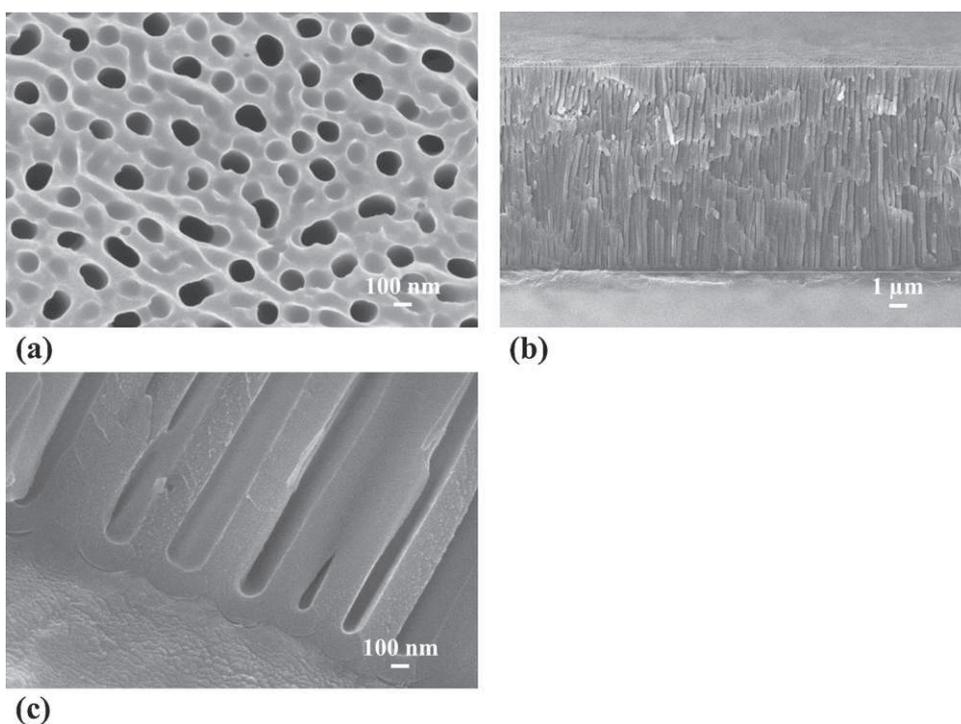
Fig. 3. FEG-SEM plan (a) and cross sectional (b, c) views of the standard porous anodic film ( $T=25^\circ\text{C}$ ,  $j=1.5\text{ A dm}^{-2}$ , duration: 29 min).
