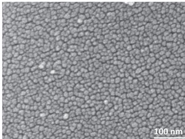
Fig. 4. FEG-SEM view of the silica nanoparticles.
