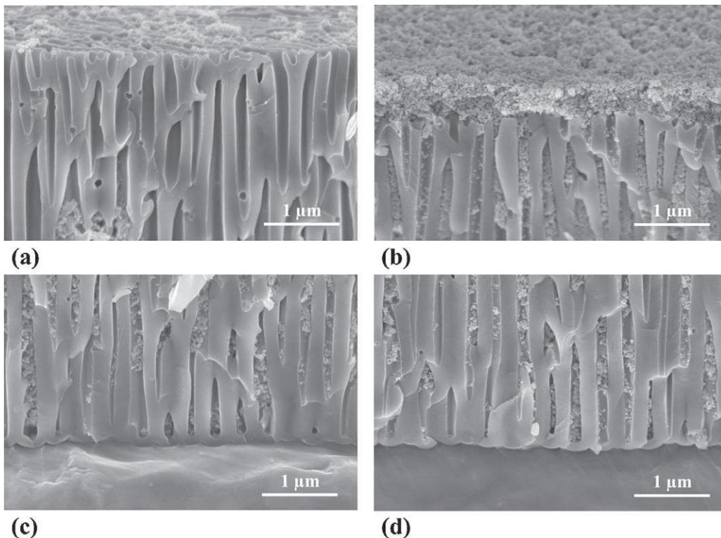
**Fig. 11.** FEG-SEM cross sectional views of the porous anodic film after the electrophoresis process using  $200\text{ V cm}^{-1}$  during 15 s (top (a) and bottom (c) of the pores) and 60 s (top (b) and bottom (d) of the pores).
