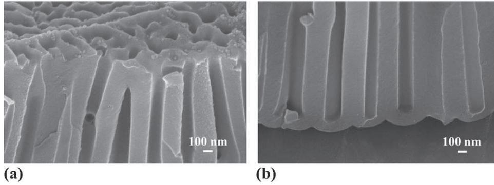
**Fig. 5.** FEG-SEM cross sectional view of the top (a) and the bottom (b) of the porous anodic film after the immersion into the suspension.
