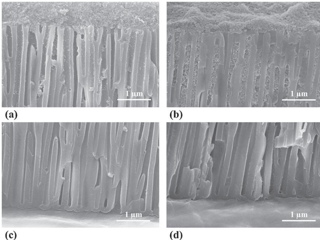
**Fig. 6.** FEG-SEM cross sectional views of the porous anodic film after the electrophoresis process using  $33 \text{ V cm}^{-1}$  (top (a) and bottom (c) of the pores) and  $200 \text{ V cm}^{-1}$  (top (b) and bottom (d) of the pores) for 5 min (suspension conductivity:  $74 \mu\text{S cm}^{-1}$ ).
