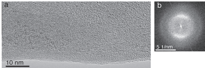
Fig. 4. (a) HR-TEM of carbon tube structures, (b) FFT image shows carbon tube graphite like spacing.
