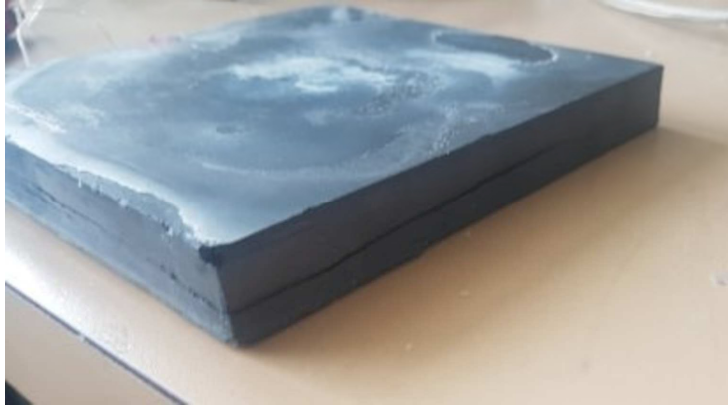
Figure 20: Cracks in the composite material after ageing.
