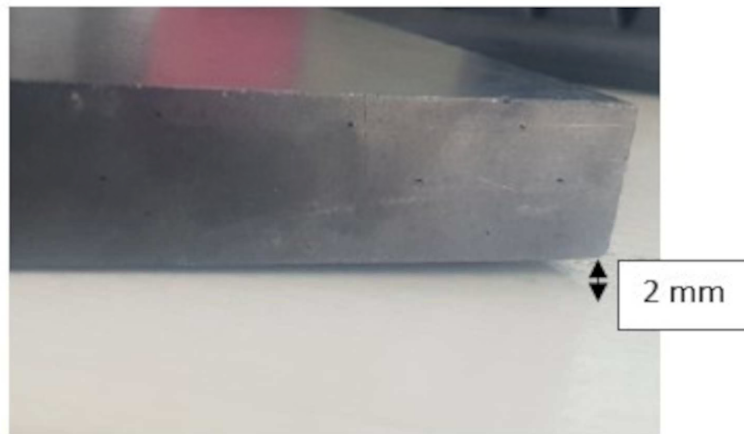
Figure 18: Composite material picture deformed after 2 cycles.
