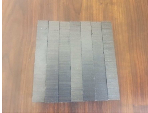
Figure 11: Composite material plate picture cut into several pieces and glued.
