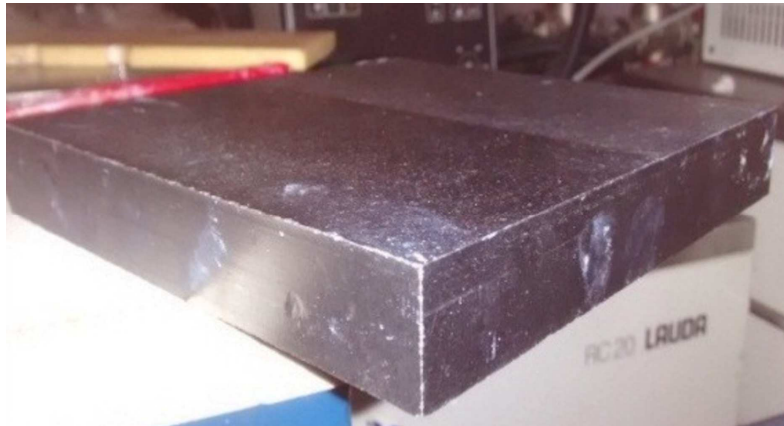
Figure 1: Picture of a CENG-PCM composite plate.
