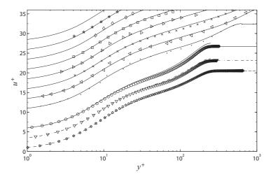
Figure 14. Zero and adverse pressure gradient boundary layer velocity profiles predicted by the interactive boundary layer model (n = 4). Symbols as in Table 1.
