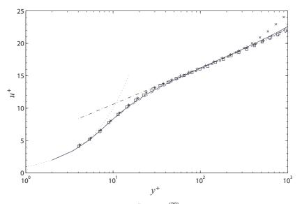
Figure 3. Inner layer velocity profiles from Österlund<sup>(20)</sup> (symbols) and from Equation 6 (lines). Inner law of the wall from (—) Musker<sup>(30)</sup>, (––) Spalding<sup>(29)</sup>, and (–·–) von Kármán<sup>(3)</sup>. (…) u<sup>+</sup> = y<sup>+</sup>. Symbols as in Table 1.
