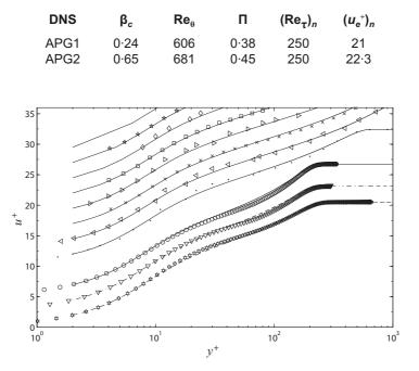
Figure 12. Adverse pressure gradient turbulent boundary layer velocity profiles fitted to Equation (6). Symbols as in Table 1.
