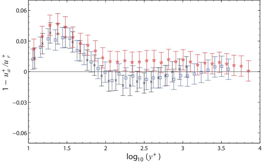
Figure 6. Percentage difference between the analytical and experimental mean velocity profiles in the wall-normal direction. Inner layer from Spalding<sup>(29)</sup>. Symbols as in Table 1.
