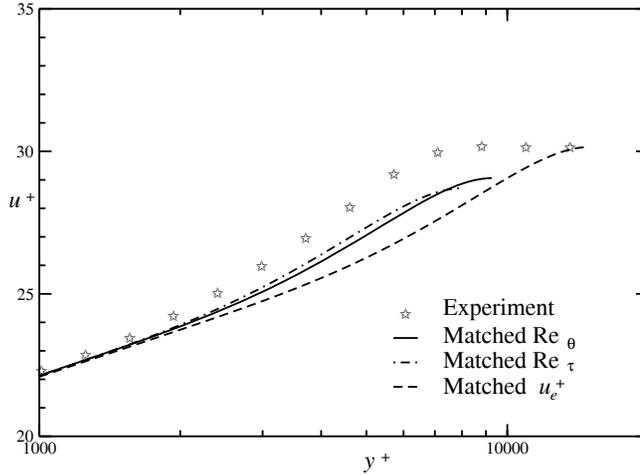
Figure 9. Outer layer profile plotted by the interactive boundary layer method.  $Re_\theta = 22,845$ .
