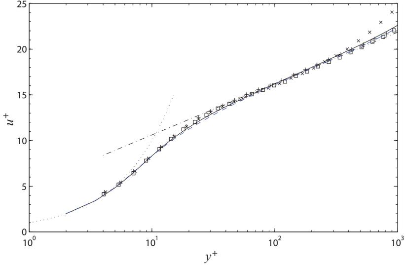
Figure 3. Inner layer velocity profiles from Österlund<sup>(20)</sup> (symbols) and from Equation 6 (lines). Inner law of the wall from (—) Musker<sup>(30)</sup>, (---) Spalding<sup>(29)</sup>, and (- · -) von Kármán<sup>(3)</sup>. (...)  $u^+ = y^+$ . Symbols as in Table 1.
