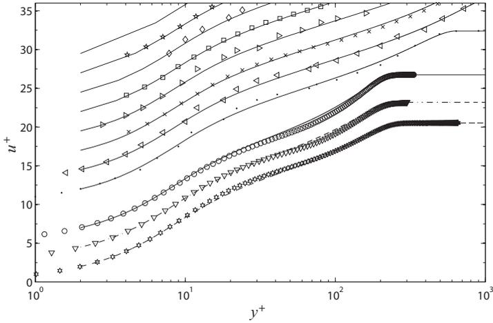
Figure 12. Adverse pressure gradient turbulent boundary layer velocity profiles fitted to Equation (6). Symbols as in Table 1.
