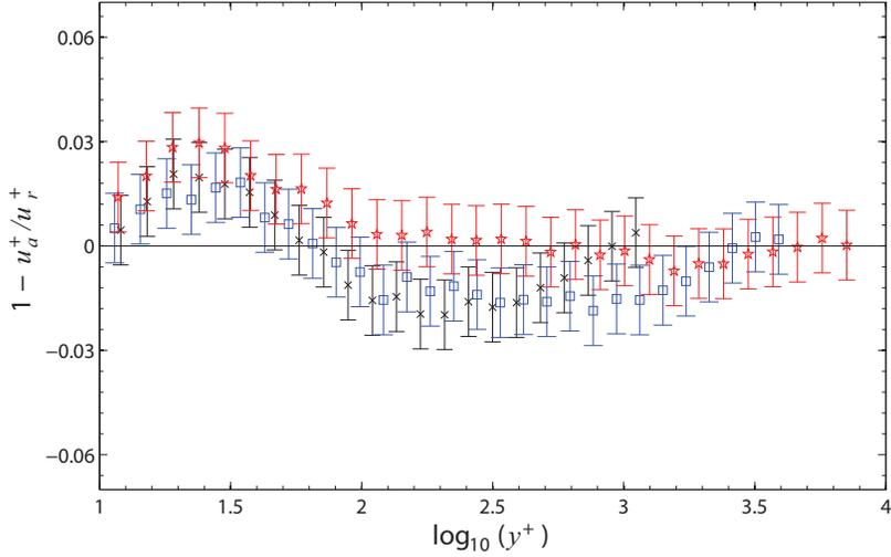
Figure 5. Percentage difference between the analytical and experimental mean velocity profiles in the wall-normal direction. Inner layer from Musker<sup>(30)</sup>. Symbols as in Table 1.
