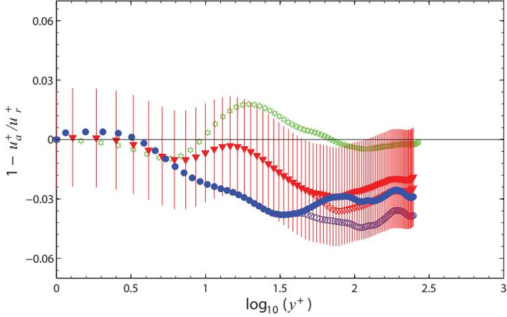
Figure 16. Percentage difference between the benchmark and the numerical velocity data in the wall-normal direction with and without adverse pressure gradient. Open symbols  $n = 4$ , filled symbols  $n = 24$ . Symbols as in Table 1.
