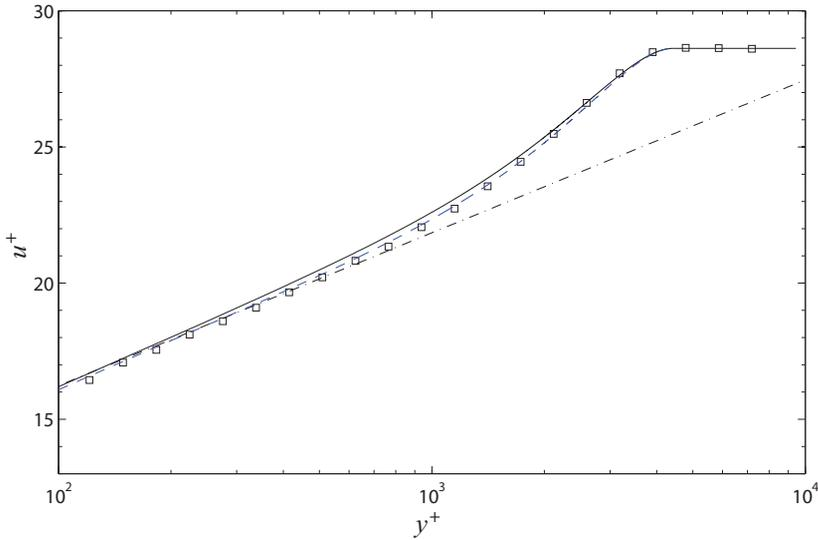
Figure 4. Outer layer velocity profiles from Österlund<sup>(20)</sup> (symbols) and from Equation (6) (lines) at. Inner law of the wall from (—) Musker<sup>(30)</sup>, (---) Spalding<sup>(29)</sup>, and (- · -) von Kármán<sup>(3)</sup>.
