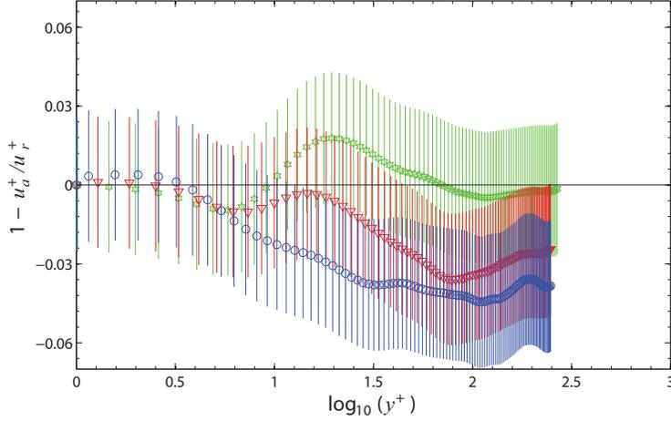
Figure 15. Percentage difference between the benchmark and the numerical velocity data in the wall-normal direction with and without adverse pressure gradient.  $n = 4$  in Equation (13). Symbols as in Table 1.
