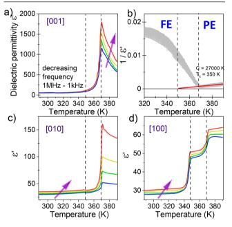
Figure 3. (a) Temperature dependence of the dielectric permittivity  $\varepsilon'$  of MHy<sub>2</sub>PbBr<sub>4</sub> measured on heating along the [001] direction. (b) Curie–Weiss dependence for the sample measured along the [001] direction. (c and d) Temperature dependence of the dielectric permittivity  $\varepsilon'$  of MHy<sub>2</sub>PbBr<sub>4</sub> measured along the [010] and [100] directions, respectively.
