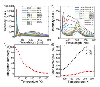
Figure 5. (a and b) Temperature-dependent PL spectra of MHy<sub>2</sub>PbBr<sub>4</sub>. (c) Temperature dependence of the integrated intensity for the FE band. (d) Temperature dependence of the band center positions for the FE and CE bands.
