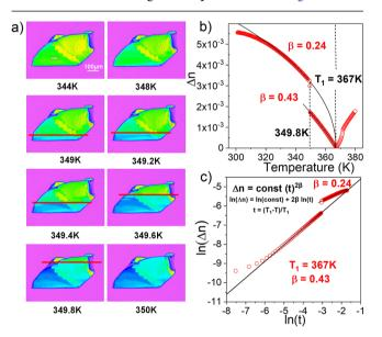
**Figure 4.** (a) Temperature evolution of birefringence maps near the transition at 350 K. a axis is perpendicular to the crystal surface, and solid line denotes the thermal front moving in the [010] direction. (b) Temperature dependence of birefringence  $\Delta n$  in the (b,c) plane. (c) Dependence of  $\ln(\Delta n)$  versus  $\ln(t)$  plotted in order to determine the exponent  $\beta$ .
