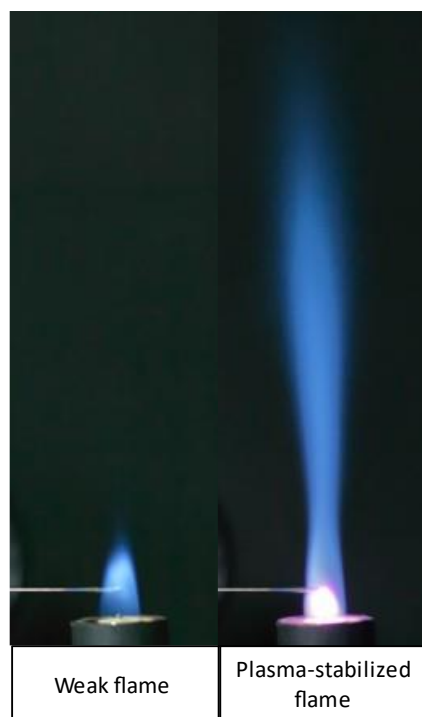
Fig. 2 Photographs of the lean flame ( \Phi = 0.8 ) without (left) and with (right) 1.8-mJ nanosecond discharges applied at 20 kHz.
