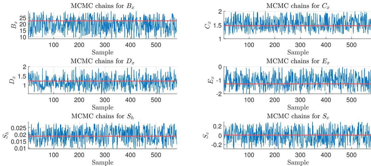
Figure 19: Traceplot of  $\theta_{MCMC}$  ( $\mu < 0.20$ ) in the case where physical prior is added. The blue curve represents the value of the samples kept. The horizontal red line indicates the reference value.
