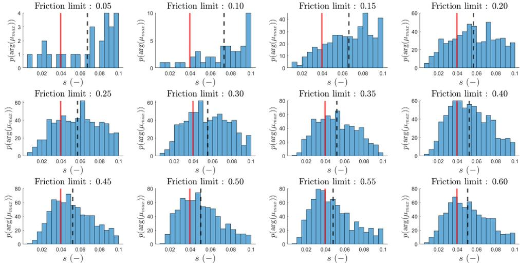
Figure 26: Evolution of the histograms representing the slip ratio corresponding to the friction potential estimated with the MCMC based estimation method with physical prior. The red line represents the reference value. The dashed black line represents the mean of the MCMC estimates.
