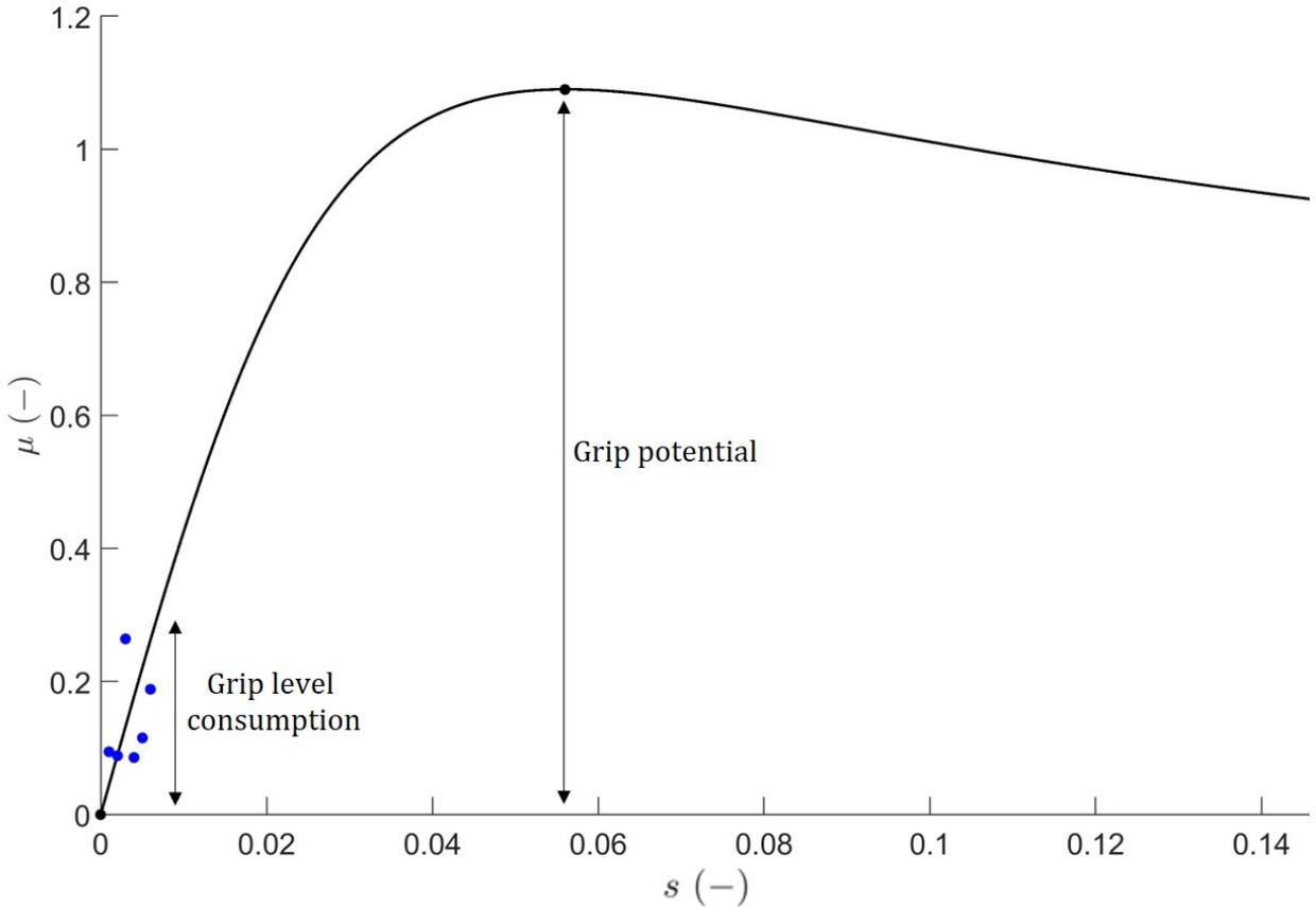
Figure 1: Example of tire friction curve. The blue points are the data points accessible under standard driving conditions.
