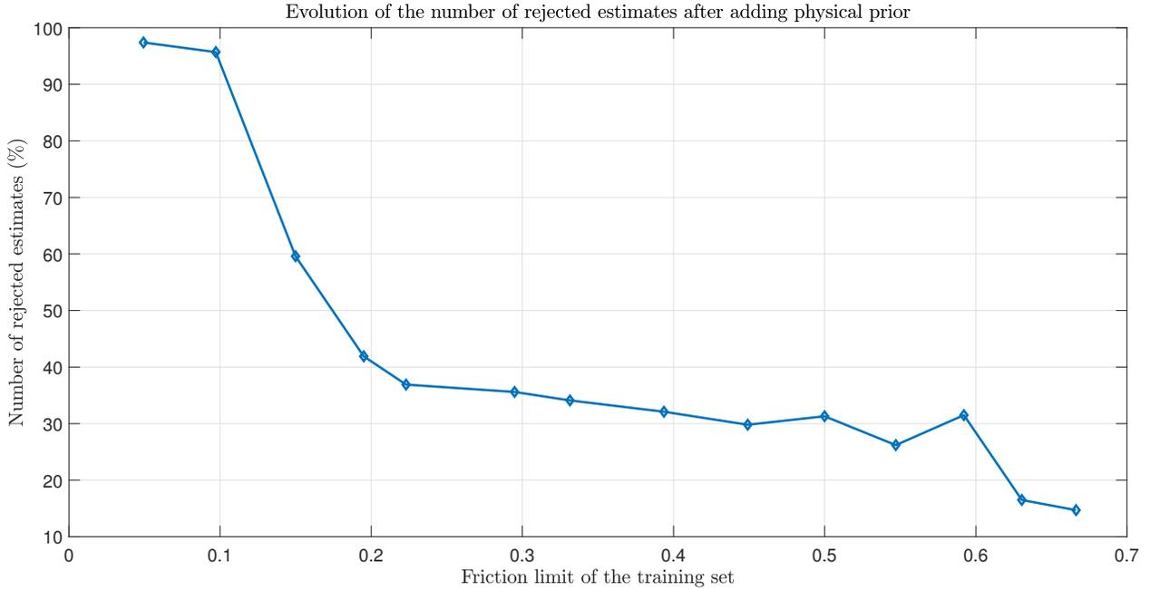
Figure 16: Evolution of the number of MCMC estimates rejected after adding physical prior.
