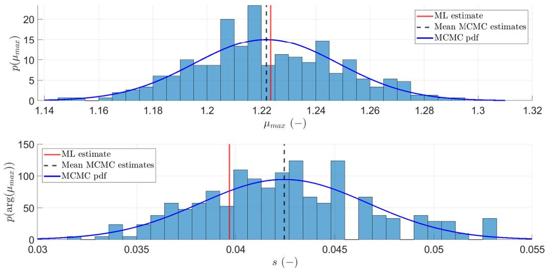
Figure 13: Histograms of grip potential estimates (upper plot) and their corresponding slip ratios (lower plot). The red line represents the values obtained with the ML method. The dashed black vertical line represents the mean of the MCMC estimates. The blue line represents a Gaussian pdf fitted to the MCMC estimates.
