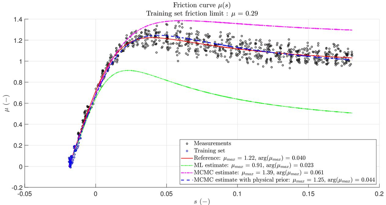
Figure 18: Results of ML and MCMC curve fitting ( $\mu < 0.3$ ). The red line represents the reference friction curve. The dashed-dot green line indicates the ML estimate. The dashed-dot magenta line indicates the MCMC estimate. The dashed blue line indicates the MCMC with physical prior estimate.
