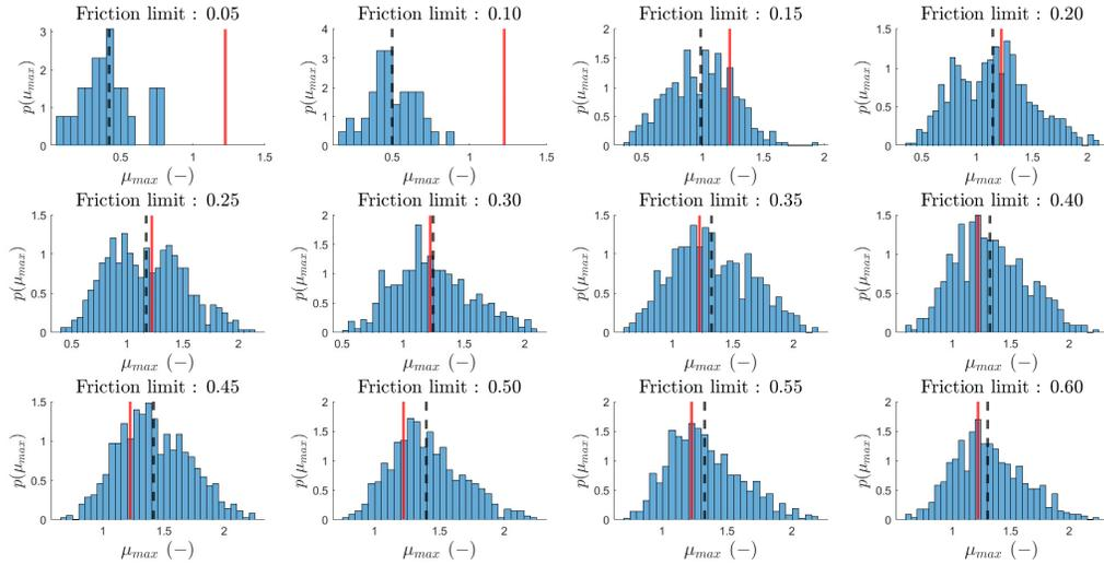
Figure 25: Evolution of the histograms representing the friction potential estimated with the MCMC based estimation method with physical prior. The red line represents the reference value. The dashed black line represents the mean of the MCMC estimates.
