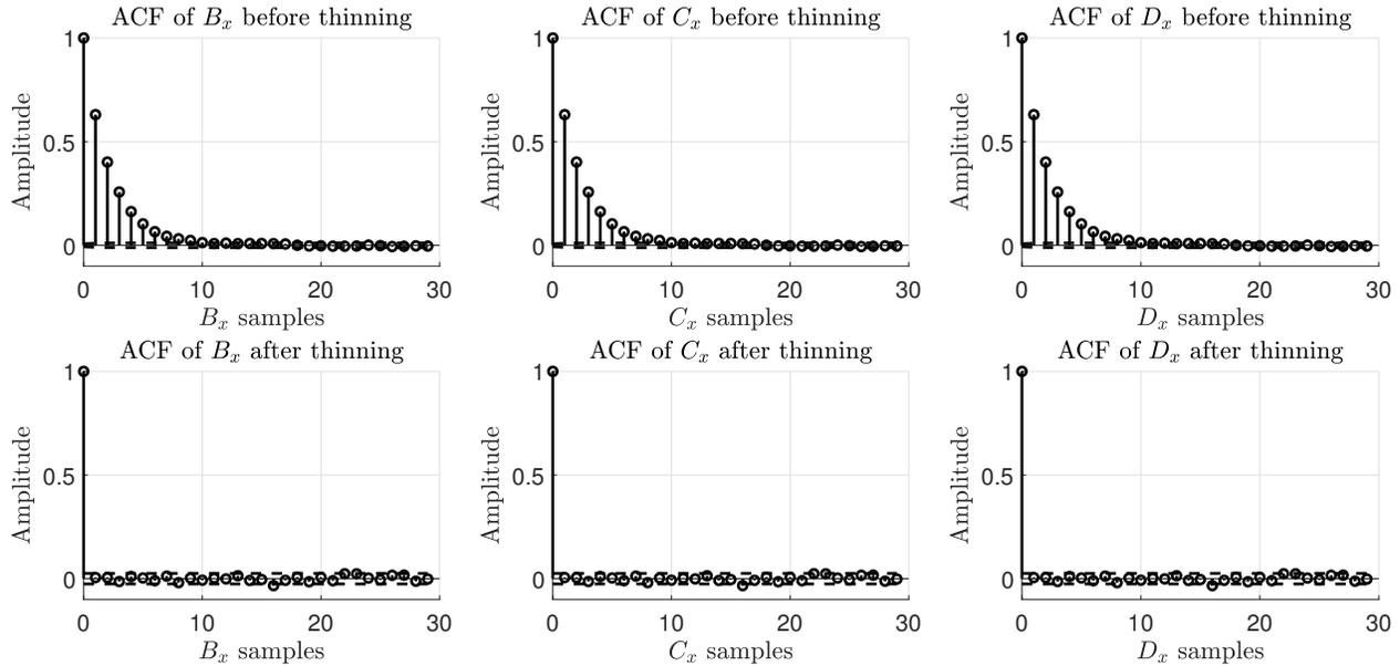
Figure 23: Autocorrelation functions of a Markov chain when the friction measurements are lower than  $\mu = 0.30$ . The upper figures represent the ACF before thinning. The lower figures illustrate the ACF after thinning. In all figures, the dashed black lines represent the standard error of the ACF with a confidence interval of 95%.
