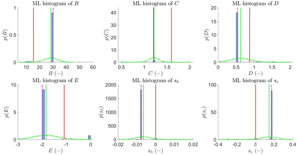
Figure 6: Histograms of the Pacejka's parameters estimated with the ML method (for  $\mu \leq 0.6$ ). The red line represents the true value used to generate the friction measurements. The green line indicates the mean of the ML estimates. The magenta dash-dot line indicates the minimizer of the loss function. The green dash-dot line represents a Gaussian pdf fitted to the 10000 ML estimates.
