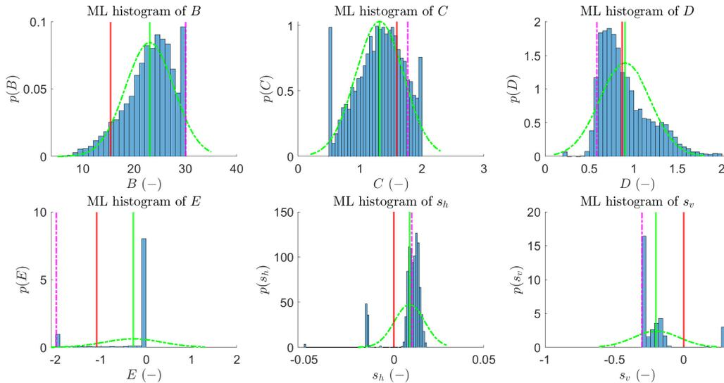
Figure 5: Histograms of the Pacejka's parameters estimated with the ML method (for  $\mu \leq 0.3$ ). The red line represents the true value used to generate the friction measurements. The green line indicates the mean of the ML estimates. The magenta dash-dot line indicates the minimizer of the loss function. The green dash-dot line represents a Gaussian pdf fitted to the 10000 ML estimates.
