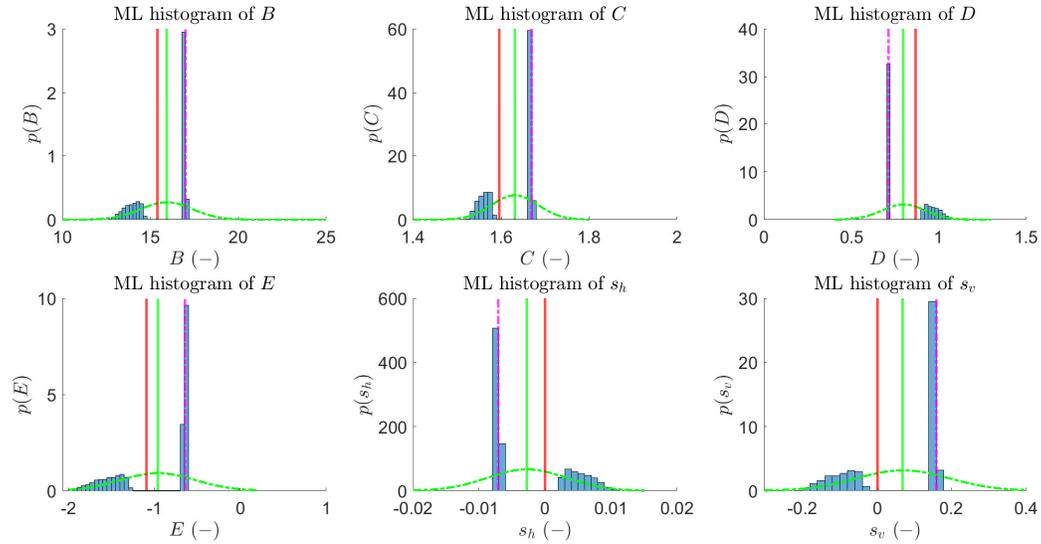
Figure 7: Histograms of the Pacejka's parameters estimated with the ML method (all data points selected). The red line represents the true value used to generate the friction measurements. The green line indicates the mean of the ML estimates. The magenta dash-dot line indicates the minimizer of the loss function. The green dash-dot line represents a Gaussian pdf fitted to the 10000 ML estimates.
