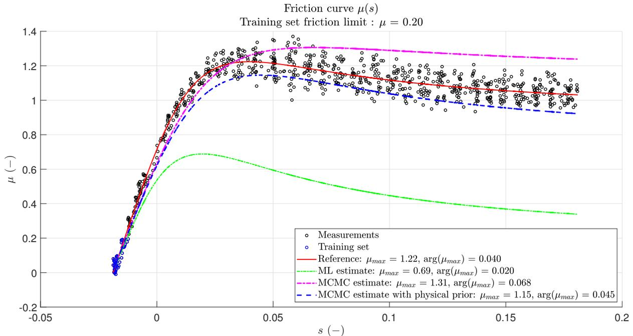
Figure 17: Results of ML and MCMC curve fitting ( $\mu < 0.2$ ). The red line represents the reference friction curve. The dashed-dot green line indicates the ML estimate. The dashed-dot magenta line indicates the MCMC estimate. The dashed blue line indicates the MCMC with physical prior estimate.
