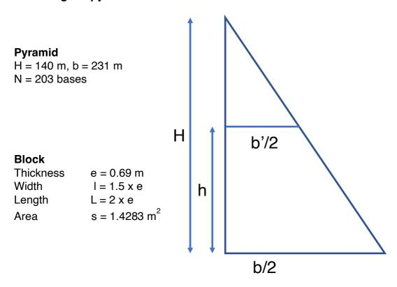
Figure 1. Half-cross section modeling the pyramid of Khufu. b is the length of the side of the base, b' the length of the side of the course at altitude h. H, is the height of the pyramid. e, the thickness of a block, which has been taken equal to the average thickness of the courses. The blocks have a width of 1.5 times the thickness and a length of 2 times the thickness. s is the floor area of a block.
