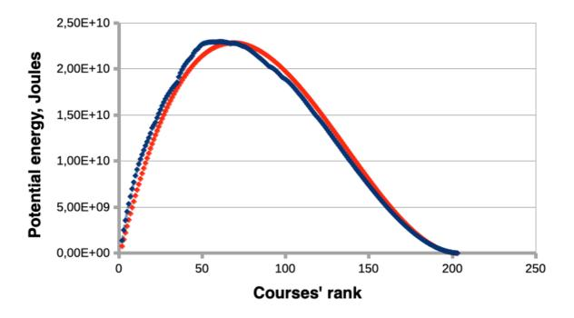
Figure 3. Gravitational potential energy of the courses: in red the theoretical curve for the model pyramid and in blue the curve obtained using the real altitude of the courses of Khufu's pyramid.
