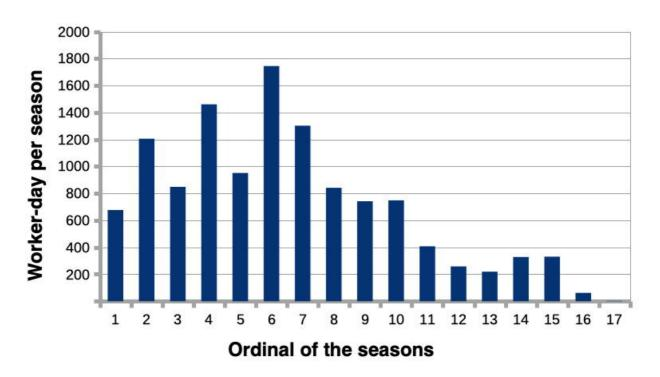
Figure 5. Total potential energy of the seasons of construction of Khufu's pyramid measured in number of working-days of 10 hours of workers developing a power of 50W.
