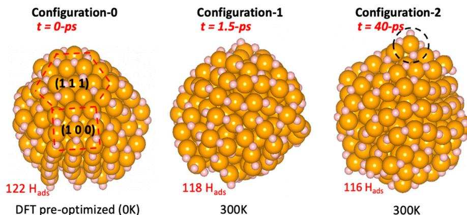
**Figure 1.** Illustration of the drastic changes in Au NPs exposed to hydrogen. Configurations extracted from AIMD simulation at 300 K, at simulation times of 0 ps (Configuration-0) where truncated octahedron initial structure was pre-optimized by DFT, 1.5 ps (Configuration-1), and 40 ps (Configuration-2). Color coding of atoms: gold in yellow and hydrogen in white. The number of adsorbed hydrogen  $H_{\text{ads}}$  is indicated in red.
