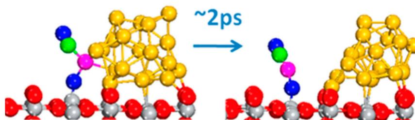
**Figure 2.** Initial (left) and successive (right) configurations sampled after 2ps during an AIMD simulation at 700 K comprising a supported Au nanocluster, one CO, and one Oad. Color coding: C: green, O: blue and red, Ti: gray, and Au: gold and pink. The pink Au atom labels the cation. Reprinted with permission from [69]. Copyright 2016 American Chemical Society.
