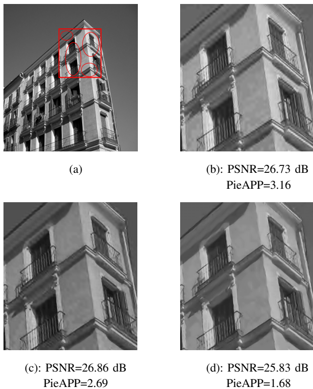
Fig. 15. (a) Original test image taken from the Tecnick-R2 dataset. Zoom on the reconstructed images at 0.1 bpp using: (b) JPEG2000, (c) CNN-LS [36], (d) D2-FCNN-LS.
