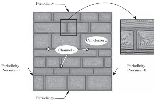
FIG. 5. Illustrations of the unit cell ( $\varepsilon_\kappa \approx 0.2$  and  $\varepsilon_\omega \approx 0.8$ ) with the mesh used for computations in COMSOL.
