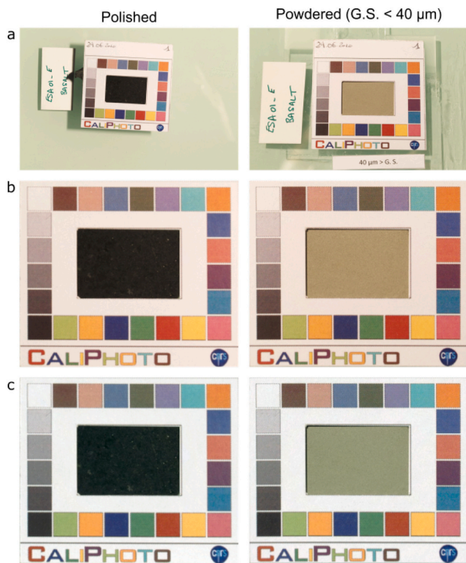
Fig. 4. Images of the ESA-01-E analogue sample, polished and powdered (G.S. < 40 μm). (a) Raw images, (b) resized images and (c) final images after CaliPhoto image processing.
