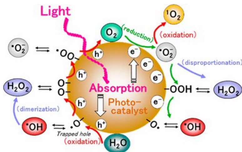
Scheme 14. Reactive oxygen species generated on the photocatalyst surface, diffusing to the surrounding aqueous medium. These reactive oxygen species are formed from the reduction of oxygen and oxidation of water and can interconvert among them. Reproduced with permission from ref. 740 Copyright 2017 American Chemical Society.
