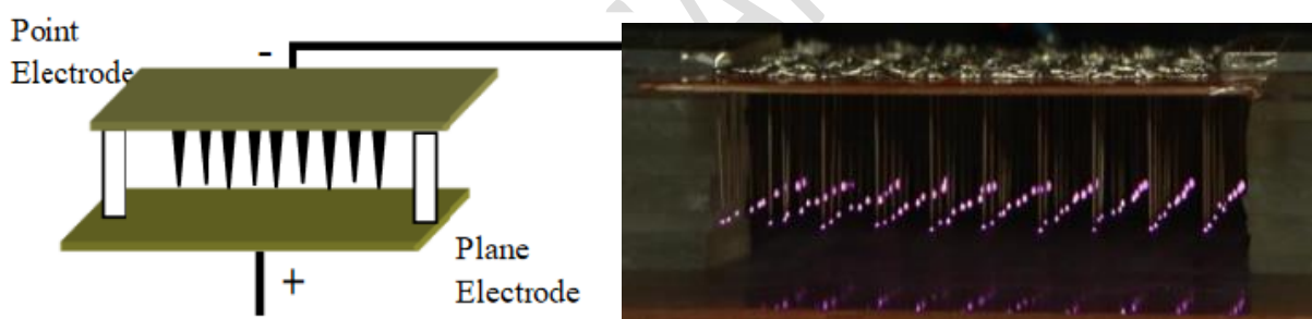
Figure 35. Corona discharge set-up. Adapted with permission from ref 290 . Copyright 2020 IOP Publishing.
