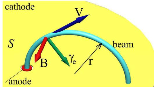
**Figure 4.** *Electron gun ejecting electrons at the velocity  $\mathbf{V}$ . A constant magnetic field  $\mathbf{B}$  bends the beam along a circular trajectory of radius  $r$ .*
