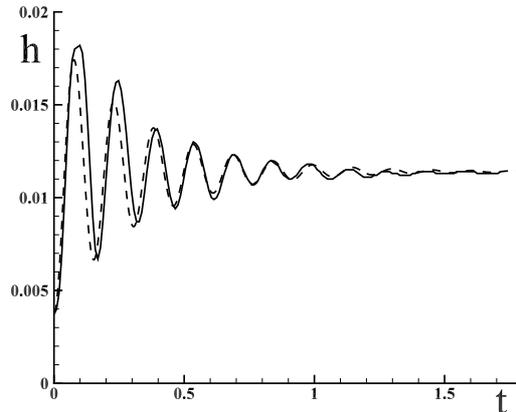
**Figure 8.** *Levitation of a cylindrical plate; height measured (solid line) [22], [23] versus computed (dash line)*
