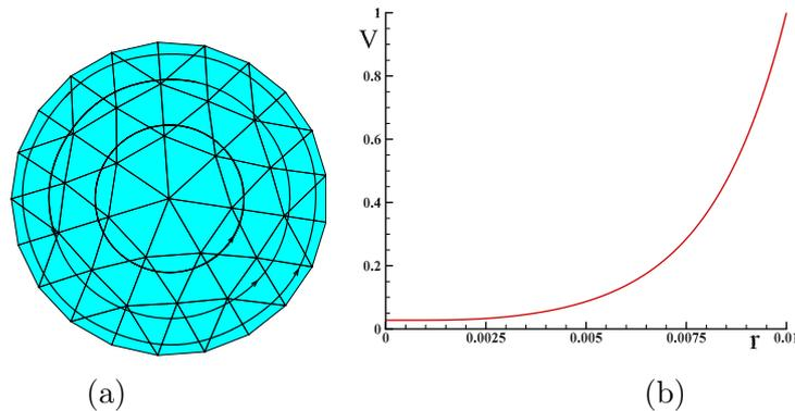
**Figure 3.** (a) Magnetic field current lines for an unstructured coarse mesh of 63 meshes based on regular triangles. (b) Reduced effective current density induced by an alternating electric current of frequency  $f$  in a cylindrical conductor.
