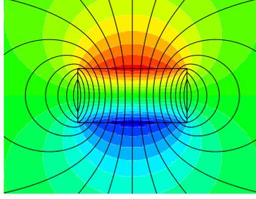
**Figure 2.** A magnet made of a ferromagnetic material represented by the rectangle produces a magnetic field on the outside. The field imposed in the magnet is equal to  $\psi^o = y \mathbf{e}_z$ . The magnetic field throughout the field is represented by a gradient of colors and the equipotentials by lines.
