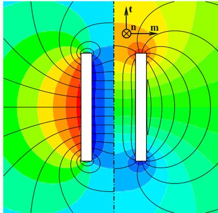
**Figure 5.** Electromagnet coil where  $\mathbf{n} = \mathbf{t} \times \mathbf{m}$  is the unit vector orthogonal to  $(r, z)$  plane;  $\mathbf{E}$  following  $\mathbf{m}$ ,  $\mathbf{B}$  ( $\psi$ ) according to  $\mathbf{n}$  and  $\mathbf{j}$  ( $\mathbf{V}$ ) following  $\mathbf{t}$
