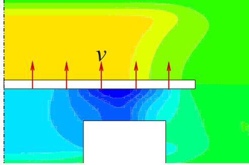
**Figure 7.** Levitation of an aluminum plate; instantaneous pressure field at time  $t = t_0 + 8 \cdot 10^{-5} s$  in the vicinity of the plate during its upward motion. The average pressure difference on either side of the plate is equal to  $\Delta\phi^o = [-35, 15]$  or  $\Delta p = [-41, 18] \approx 60 Pa$ .
