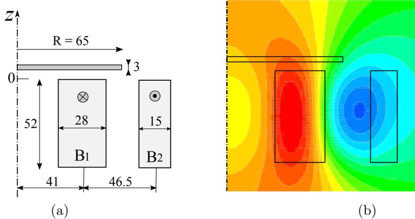
**Figure 6.** *Levitation of a cylindrical plate; (a) electrodynamic levitation device with dimensions in mm; (b) average scalar potential  $\bar{\phi}^o(r, z)$ .*
