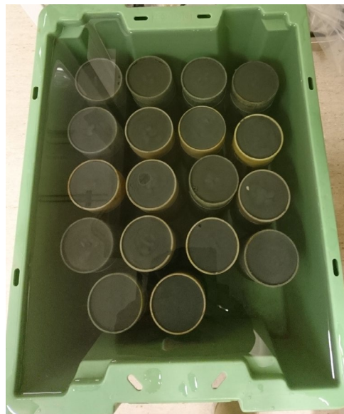
Figure 1. Photo showing specimens (sediments stabilized by cement in various proportions) cast in sampling sleeves stored in the water bath. Photo by Per Lindh.
