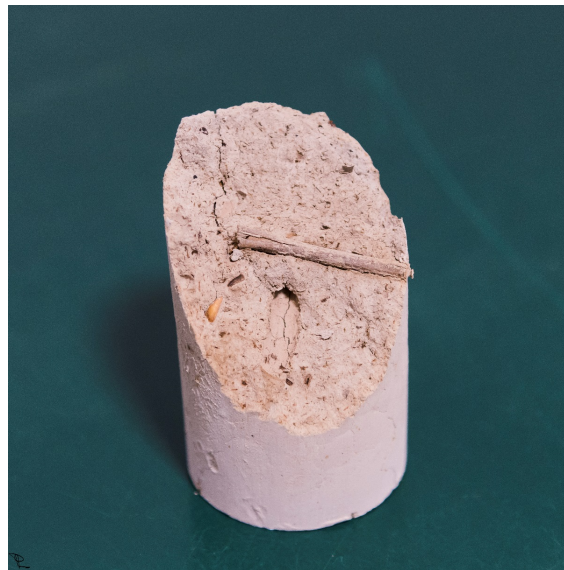
Figure 3. Photo showing fracture surface of the stabilized specimen. Note the reed piece directly exposed in the fracture plane. Photo by Per Lindh.
