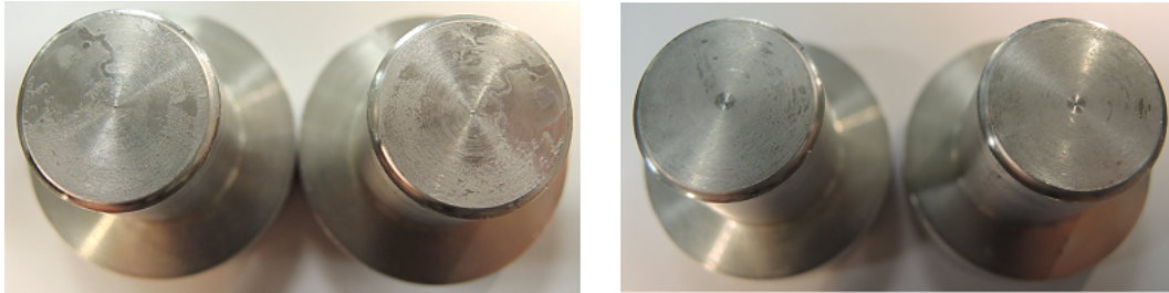
Figure 28: Fracture facies observed on Cyanoacrylate joint after an impact test in traction.
