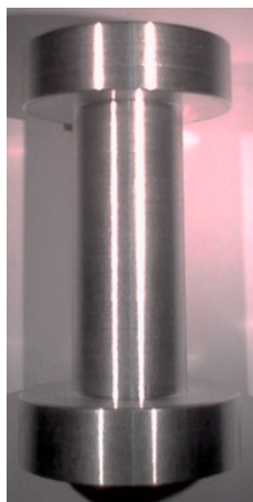
Figure 5: One-piece specimen without the adhesive joint.
