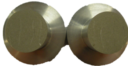
Figure 26: Fracture facies observed on Araldite joint after an impact test in traction.
