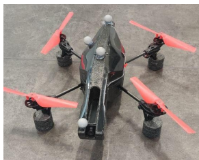
Fig. 5: Aerial drone used during experimental tests. Some reflective markers were put on the drone to be recognised by the OptiTrack camera system
