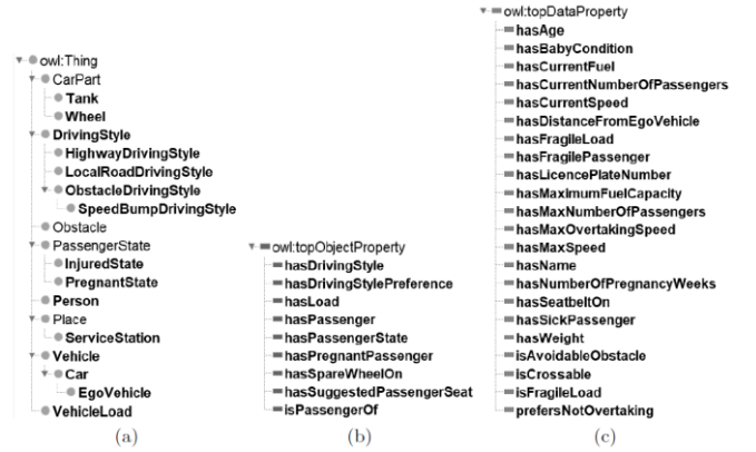
Figure 3. Modelling the context of navigation with. (a) Classes; (b) Object Properties; (c) Data Properties.
