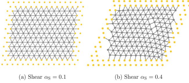
FIG. 6. (Color online) Sequence of events corresponding to a shear deformation applied to a non-Brownian cell population ( $15 \times 15$  cells) described using model 1 for (a)  $\alpha_S = 0.1$  and (b)  $\alpha_S = 0.4$ . The CBR is valid in the limit of small deformations and fails if  $\alpha_S$  exceeds a critical value (here  $\alpha_S \sim 0.2$ ) at which strains in the narrowed corners become large enough.
