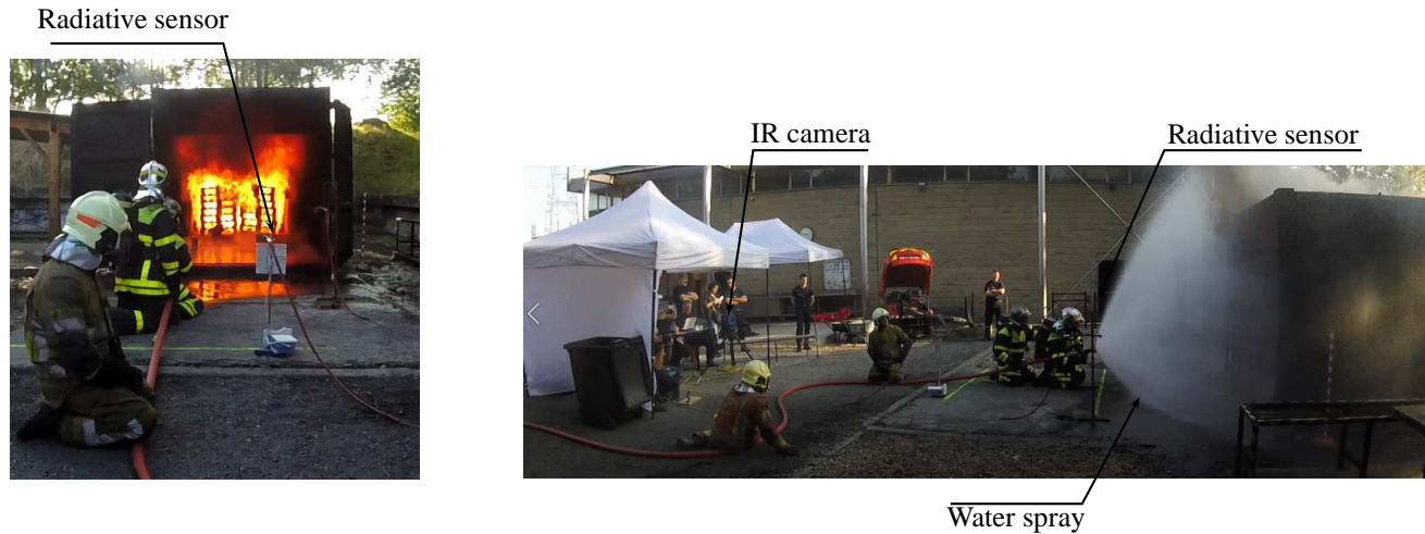
(a) Rear view of the experimental set-up without water spray activation
