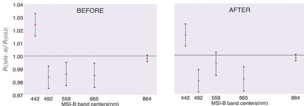
**Fig. 5.** The intercomparison of OLI and MSI-B  $\rho_t$  products before (left) and after applying vicarious corrections using preliminary gains (Table 1) for the visible and the 865-nm bands. The data points represent median values of MSI-B to OLI ratios computed from 24 scene pairs collected at n-SNO events. The error bars represent one-standard deviation. Note that the NIR band has not been vicariously adjusted.
