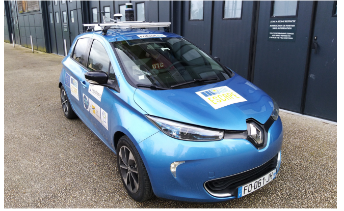
Fig. 3: Experimental vehicle of the Heudiasyc laboratory used in these experiments. It is equipped with a low-cost GNSS receiver, a Mobileye camera, and a Velodyne VLP-32C lidar. Ground truth is provided by a post-processed IMU with PPK GNSS.
