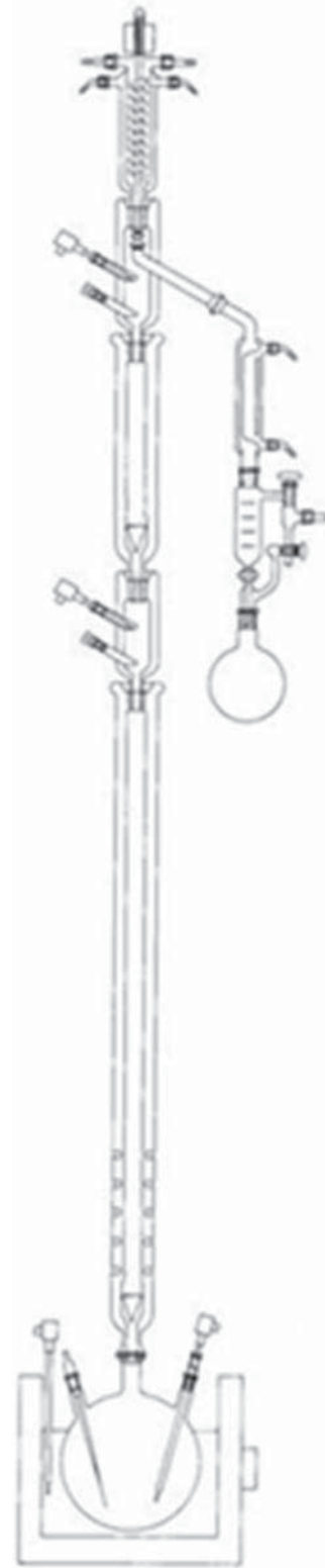
Fig. 3 – Batch distillation column configuration at laboratory scale.
