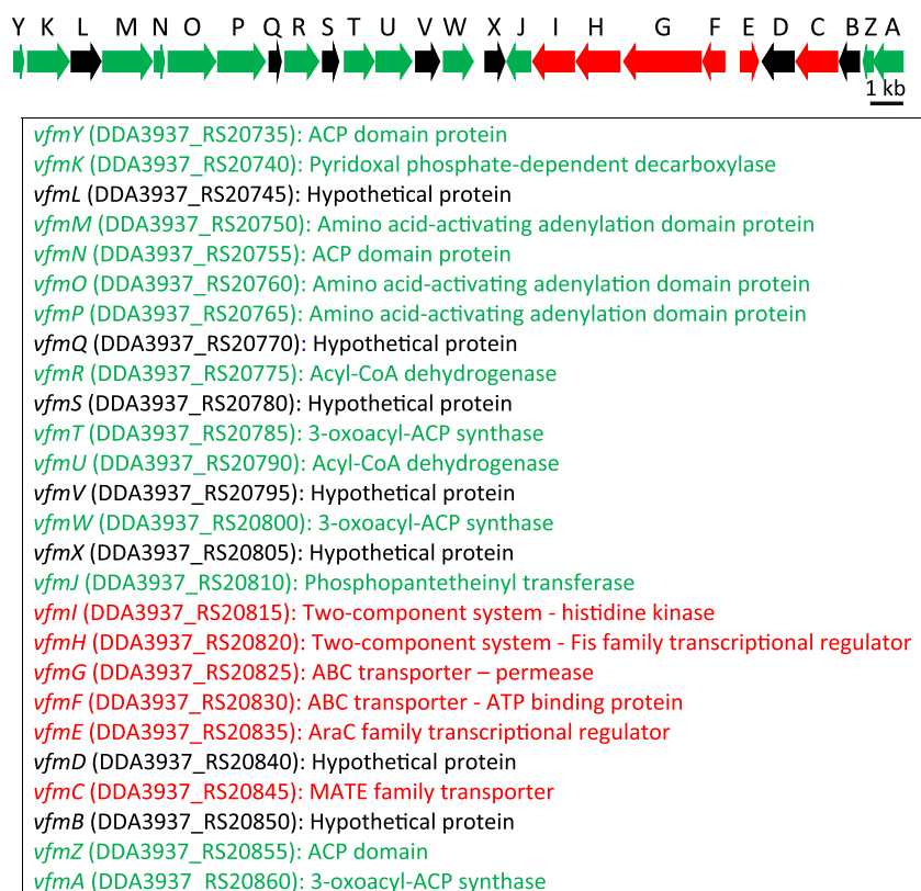
Fig. 1. Functional annotation of the vfm gene cluster of Dickeya dadantii 3937 (taken from the GenBank accession NC_014500). In the upper part, the 26 genes of the gene cluster are presented by arrows. Green arrows correspond to genes annotated as biosynthesis genes, red arrows are for genes annotated as regulatory or transporter genes and black arrows for genes encoding hypothetical proteins. The length of arrows is proportional to the gene length according to the scale indicated at the right. The predicted function of each gene is shown below, with the same colour code. Abbreviations: ABC: ATP binding cassette, ACP: acyl carrier protein, MATE: multidrug and toxic compound extrusion. The corresponding GenBank tags are indicated for each vfm genes.
