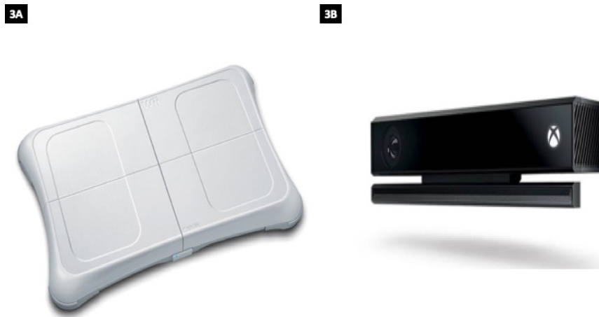
Fig. 3: Sensors used to assess posture in ASD: Nintendo Wii balance board™ (A); Kinect™ (RGB-D sensor) (B).
