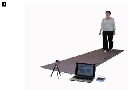
Fig. 4: The clinical stride analyser® (B & L Engineering, CA, USA)
