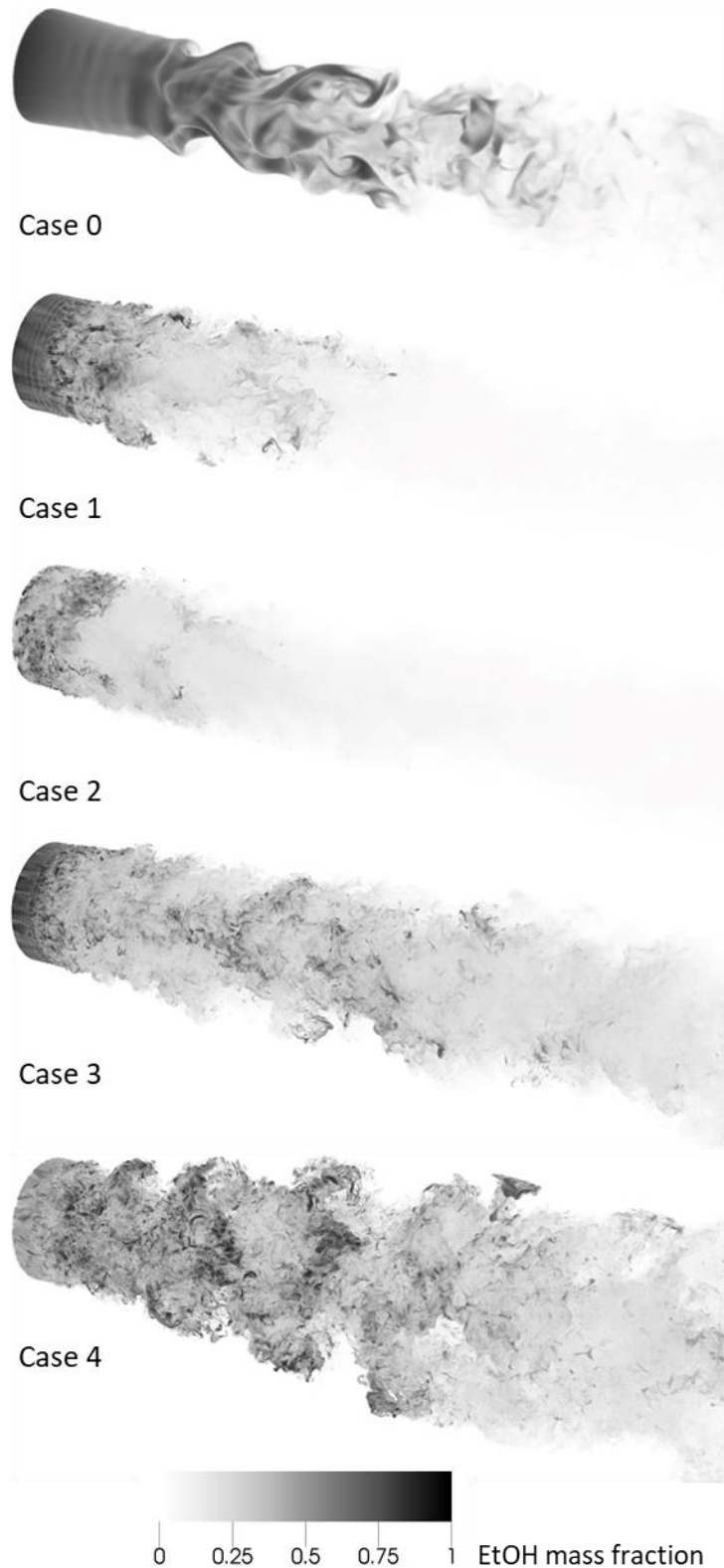
Fig 4. Instantaneous concentration volume renderings for the cases 0 to 4 (top to bottom) - see additional videos 2-6. The turbulent transitions of the coaxial jets is due to the significant development of primary and secondary Kelvin-Helmoltz instabilities resulting from strong shear stress between layers of different densities. DNS emphasizes the multitude of scales and highlights the
