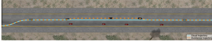
Fig. 16 The GRNDriver avoids the red car. The plain line is the normal trajectory, the dotted line is the altered trajectory using a 2.65 factor on the right track sensor used to position the car in the middle of the track (Color figure online)
