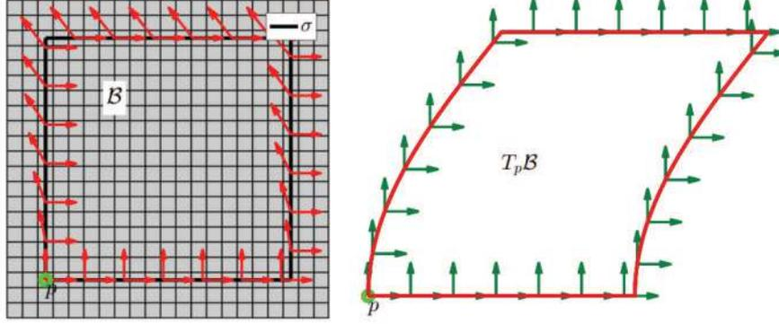
**Figure 5.** Left: The same defect-free current state as in Figure 4 but represented in  $\mathcal{B}$ . Right: Developing curve  $\tilde{\sigma}$  of  $\sigma$  on  $T_p\mathcal{B}$ .
