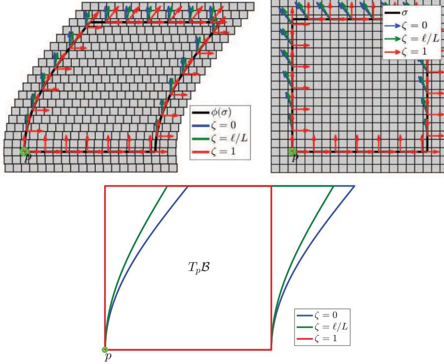
**Figure 7.** Numerical simulations of the transformation (44). The current state has no torsion and no curvature but the metric is not compatible with the induced connection. Top representation in  $\mathbb{E}^3$  (right) and in  $\mathcal{B}$  (left). The frame at  $p$  is parallel-transported along  $\sigma$ . The bottom developing curve of  $\sigma$  on  $T_p\mathcal{B}$  obtained for various  $\zeta$ .
