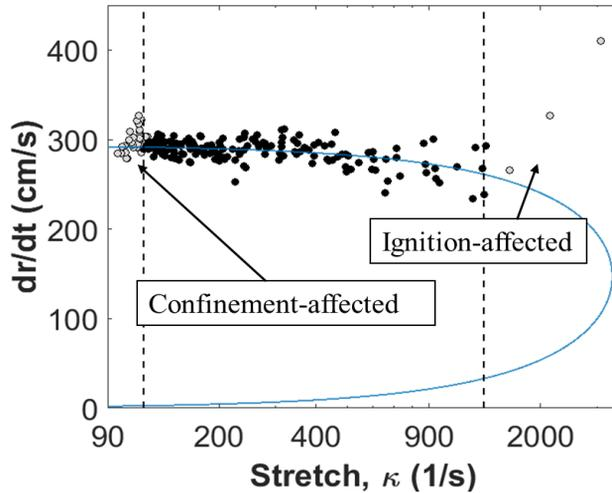
Fig. 4. Example of nPCH/air laminar flame speed determination from the stretched, burned-gas velocity (i.e.,  $dr/dt$ ) from a TAMU laminar flame experiment at  $T_i = 403$  K,  $P_i = 1.01$  bar,  $\phi = 1.34$ .
