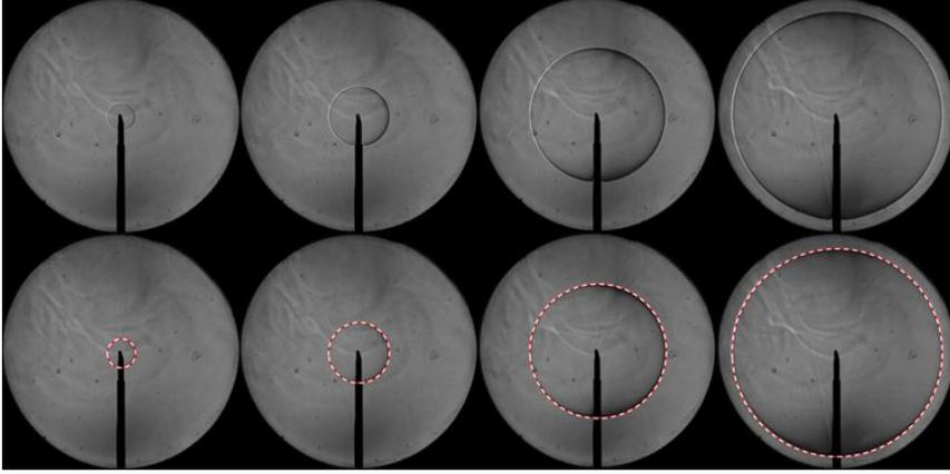
Fig. 3. Example of nPCH/air spherically propagating flame from a TAMU experiment at  $T_i = 403$  K,  $P_i = 1.01$  bar,  $\phi = 0.87$  along with edge detection (lower images) using an in-house Python code.
